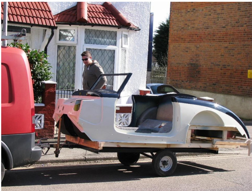
Fig.4 Body tub on the way back from the painter on its custom built trailer
